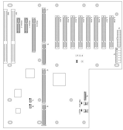
8 PCI slots : S-PCI1 ~ S\_PCI8 Remarks : 32 bits /5V by bridge.
