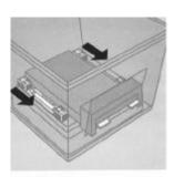
Be sure that the side of the film holder with the dark slide or focusing panel (f) faces this opening. With the film holder in place, slide the bars back to the "lock" position, in the direction indicated by the arrows in the illustration. When the film holder is properly mounted, the bars fit into the grooved edges of the film holder, securing it to the base.
