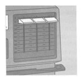
The Daylab 35 Plus enables you to adjust the color balance of your enlargement by adding amounts of the three primary colors: cyan, magenta and yellow (singly or in combination) to your print.
