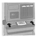
Set the VIEW-OFF-PRINT switch (1) at VIEW: the viewing light inside the enlarger head should now be on.
