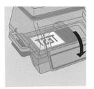
Notice that the slide carrier does **not** lock into position in the slide carrier slot, allowing you to move it in any direction to crop and center the projected image For more information on composing your picture, see *Tips for better enlargements* on page 14 of this manual.
