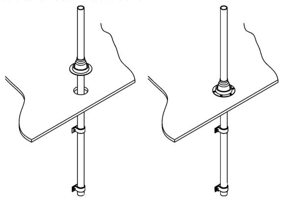
Seal the layers of roofing material to each other with a silicone caulk or sealant so that moisture is prevented from penetrating through to the wood. Apply a generous amount of sealant to the base of the seal. Slide the seal the rest of the way down onto the roof and locate it so that the base is centered over the hole.
