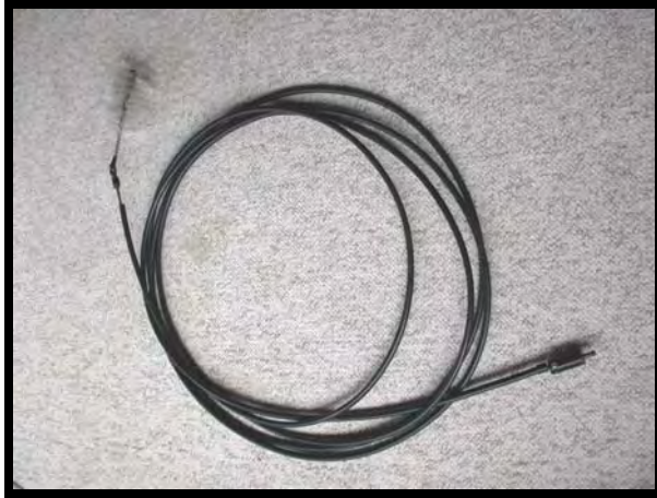
Pipe cleaning brush and "snake"
