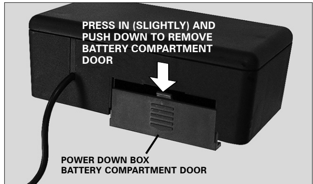
FIGURE 2: Power down box battery compartment door removal.
