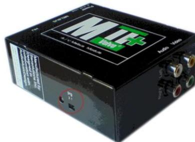
Figure 4 Switch location on an MII+
