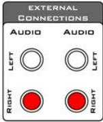
With the MII you are able to integrate 2 additional stereo audio sources to your HU. This is possible through 4 RCA jacks (2 stereo channels) located on the side of the device. Through firmware updates you can choose on which source you would like to run the MII: The external 10 CD Changer, MD Changer (not applicable for all HU's), Television or Satellite Receiver (only on HU-x50 units).
