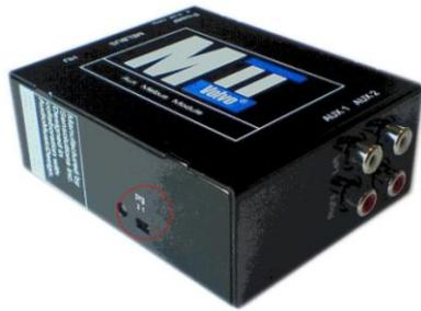
Figure 3 Switch location on an MII
