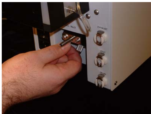
Figure 2-1 Location of WCPC Wick on Sample Inlet Assembly
