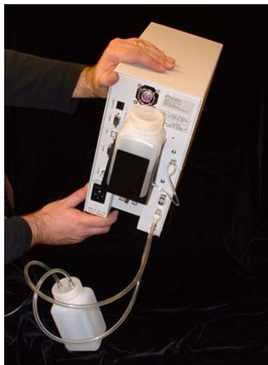
Figure 2-5 Tipping the WCPC During Drain Cycle for More Complete Drain of the Reservoir
