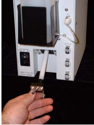
Figure 2-2 Installation of WPCPC Wick on Sample Inlet Assembly
