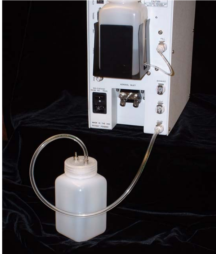
Figure 2-4 Drain Bottle Connection
