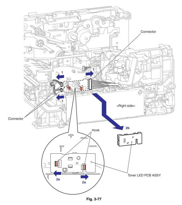
(3) Release the Hook to remove the LED holder from the Toner LED PCB ASSY.
