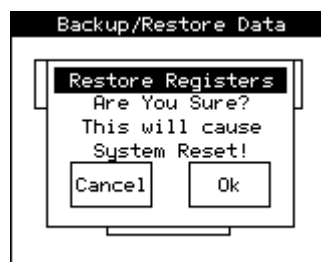
Figure 15-4 – Restore OCS Data
