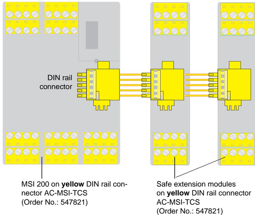
Figure 2-2 TBUS DIN rail connector from Leuze electronic
