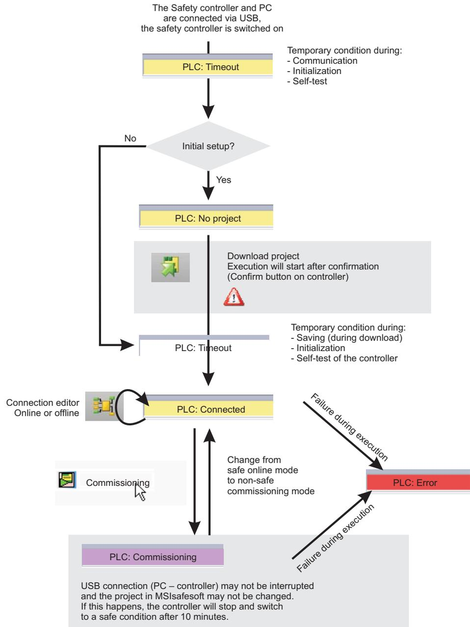
Figure 3-3 Possible operating modes (status) of the safety controller
