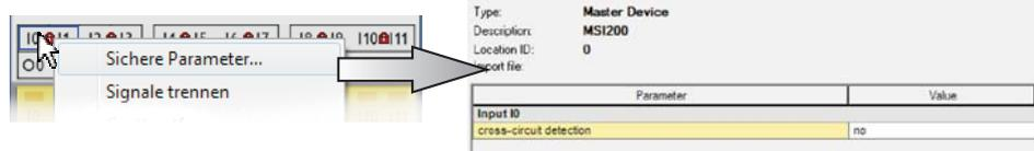
Figure 5-13 Opening the parameterization editor via the context menu
