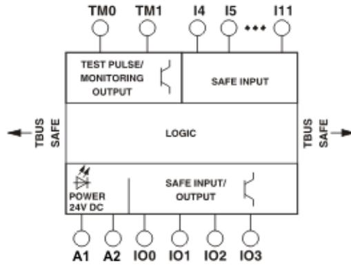
Figure 4-2 Block diagram MSI-EM200-8I4IO
