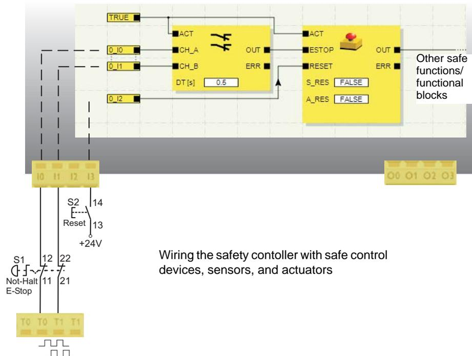
Figure 2-4 Implementing cross-circuit detection for an emergency stop control device at inputs I0 and I1 of the safety controller
