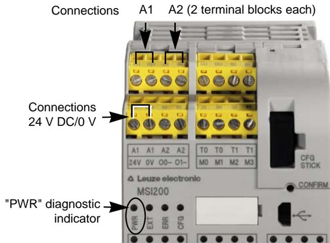
Figure 3-11 Connecting the supply voltage at A1/A2 and 24V/0V
