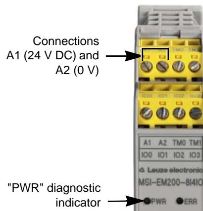
Figure 4-5 Connecting the supply voltage
