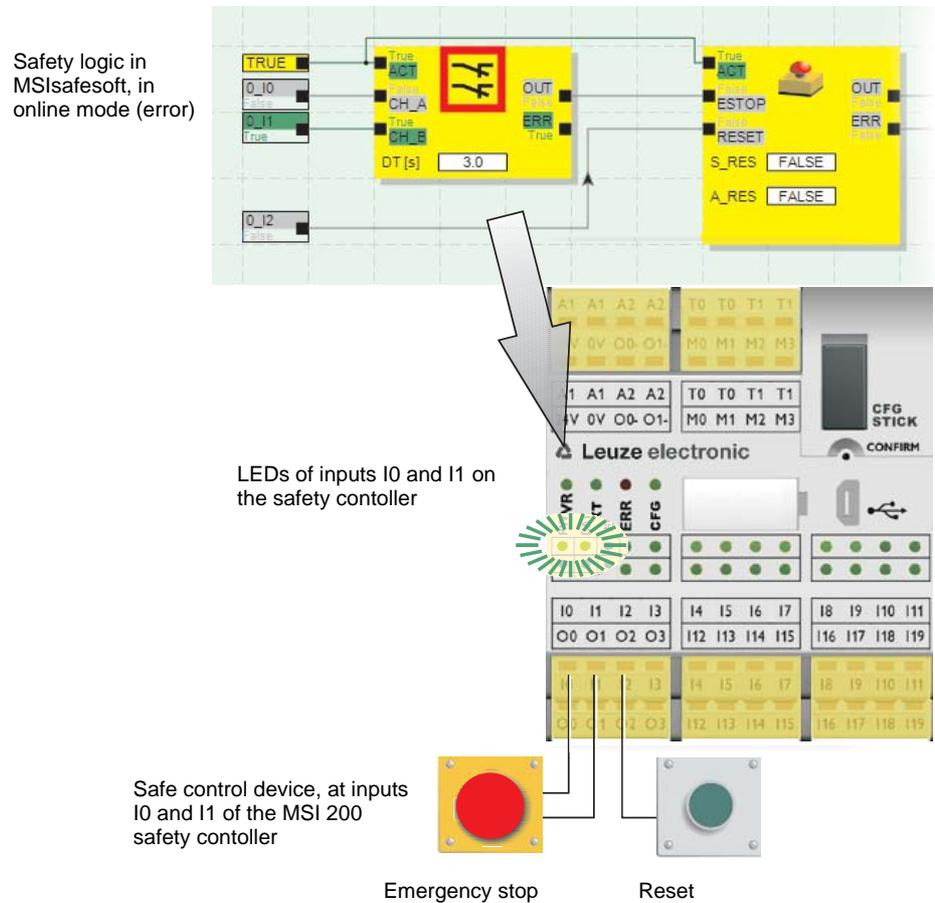
Figure 2-6 Hardware diagnostics in the event of a safe functional block error
