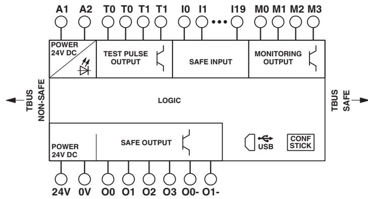
Figure 3-2 Block diagram of the MSI 200 safety controller
