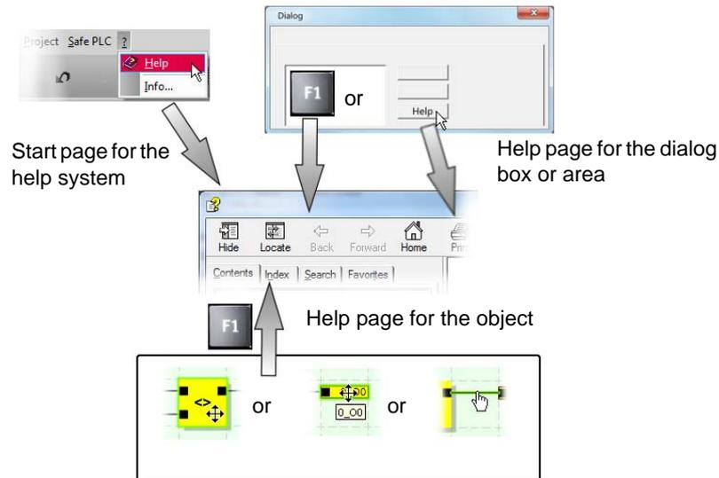
Figure 1-1 Calling the online help in the configuration software MSIsafesoft
