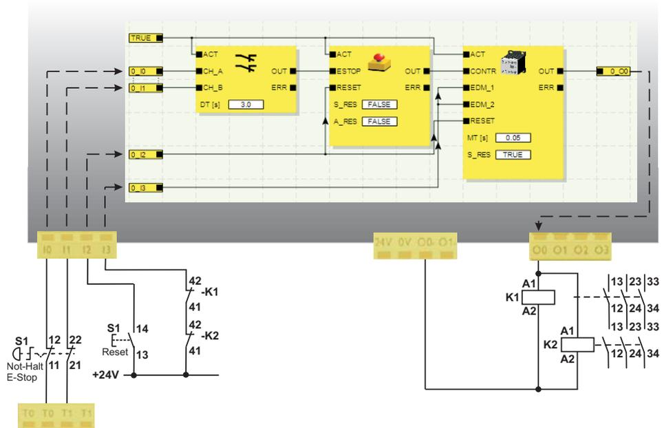
Figure 3-6 Example application for grounded switching outputs O0- and O1-
