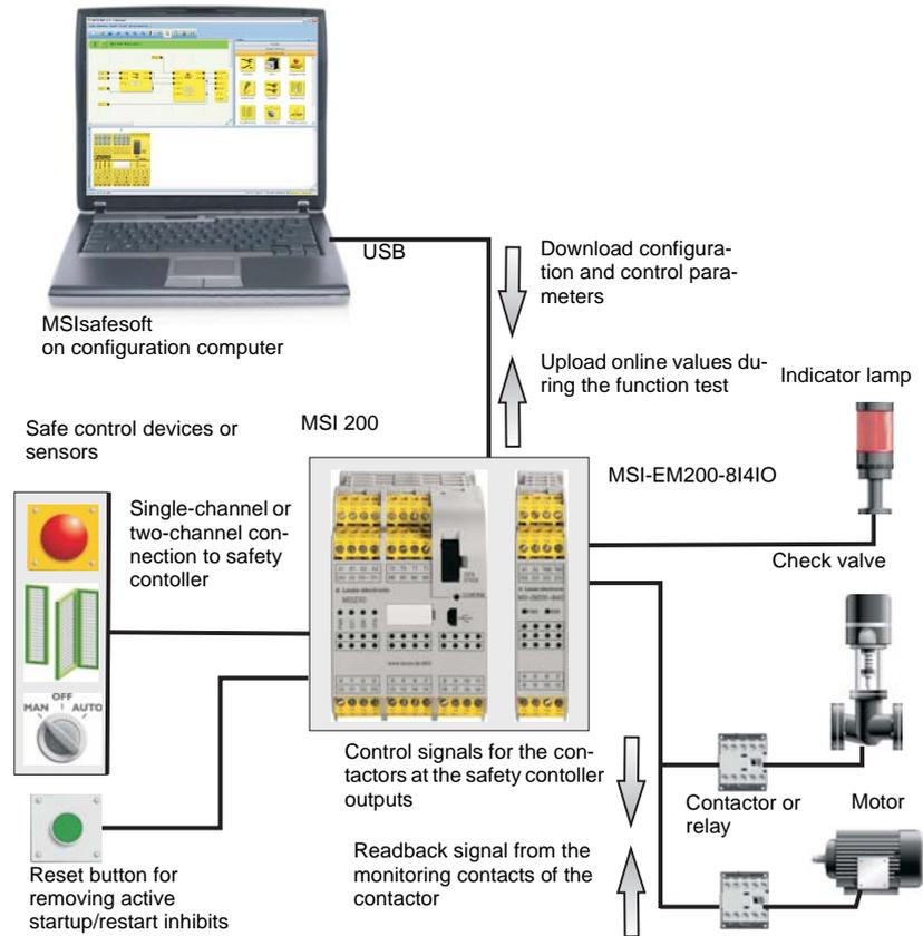
Figure 2-1 Example safety system structure
