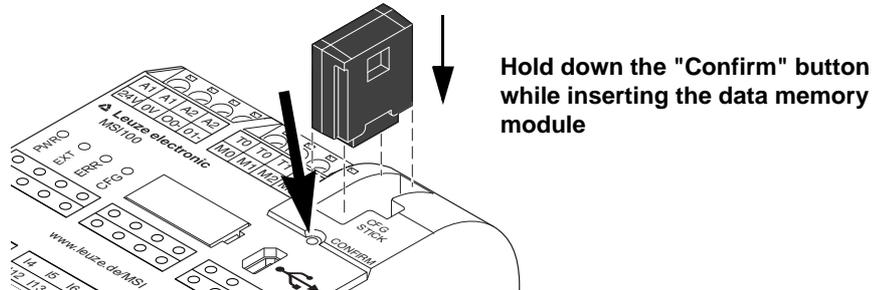
Figure 6-7 Inserting the data memory module
