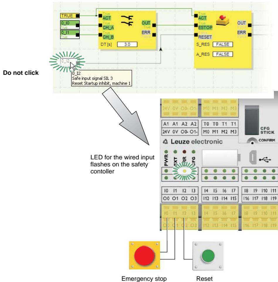
Figure 2-7 Simplified schematic view: Wiring check
