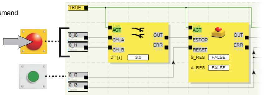
Figure 6-8 Example of a function test for the safety system using MSIsafesoft online mode
