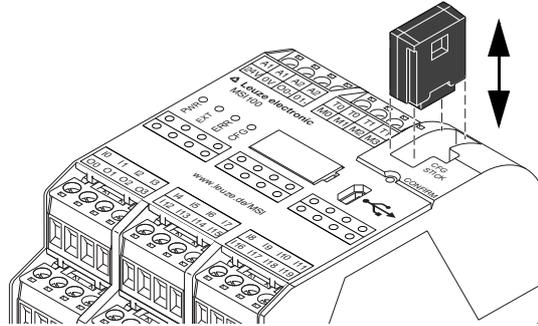
Figure 3-8 Data memory module AC-MSI-CFG1 on MSI 200
