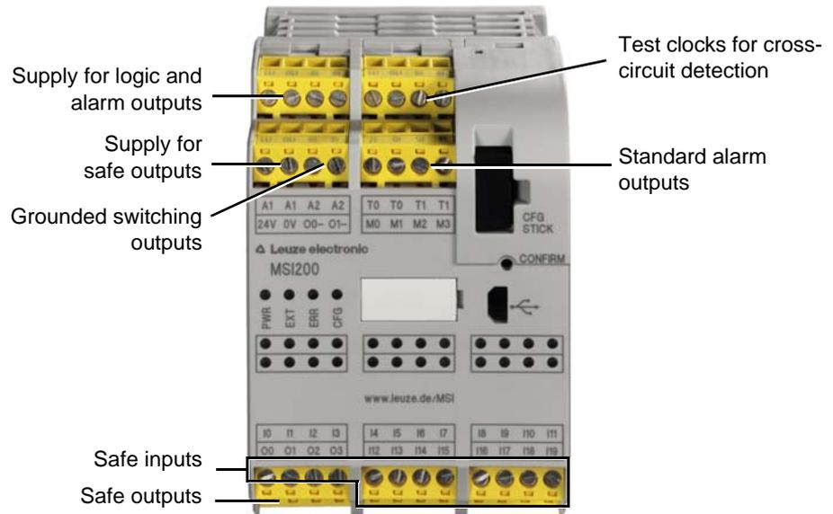
Figure 3-5 Signal connections MSI 200
