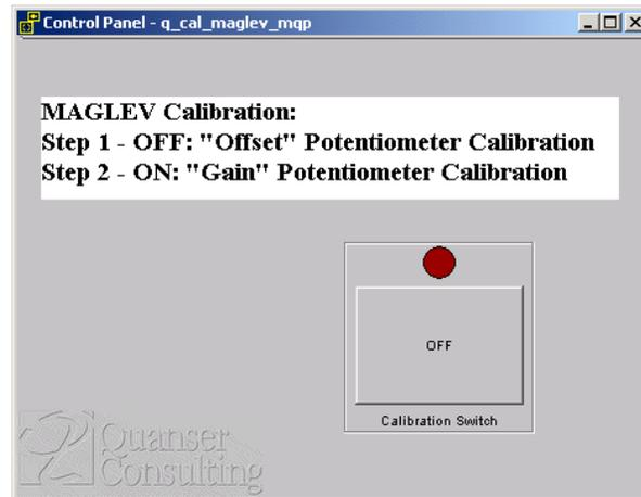
Figure 13 WinCon Calibration Control Panel
