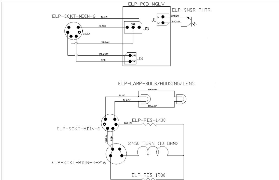
Figure 4 MAGLEV System Wiring Schematic
