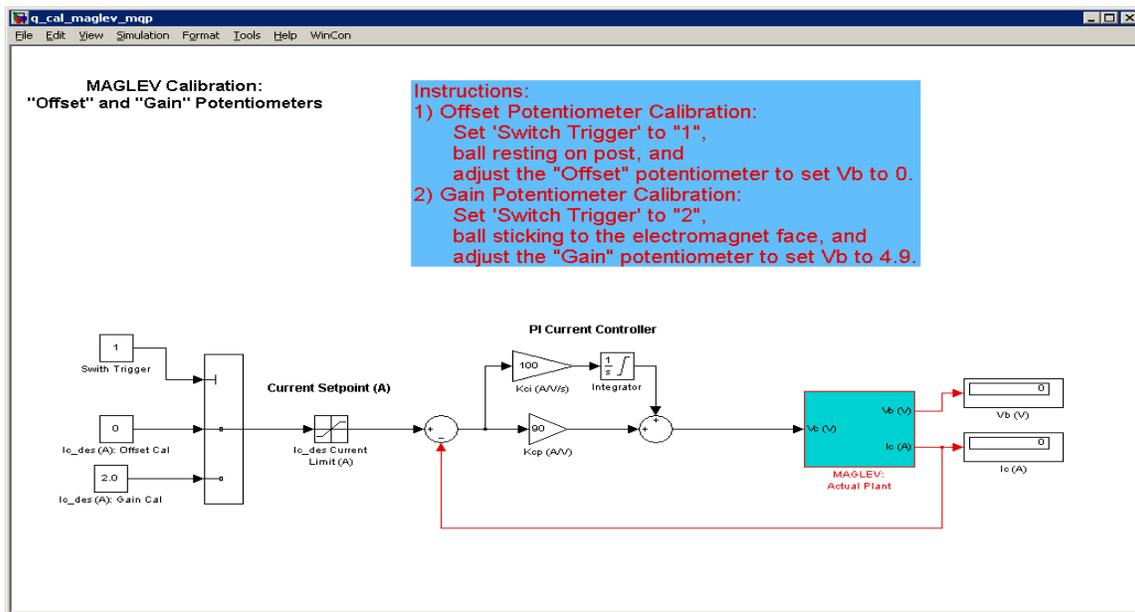
Figure 12 Position Sensor Calibration Diagram
