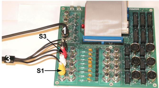
Figure 9 MultiQ-PCI Terminal Board Connections
