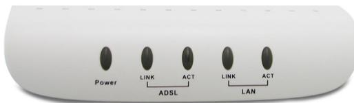
Figure 2-2 Front Panel Display with LED Indicators
