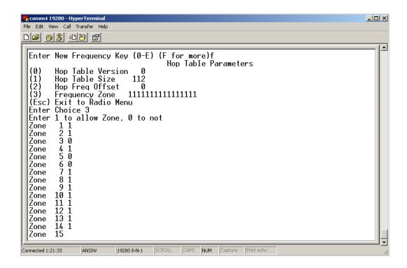
**WARNING:** FCC regulations require a minimum of 50 separate channels be used within a hop pattern. Use the above table to determine the number of frequency zones are required for legal communication.
