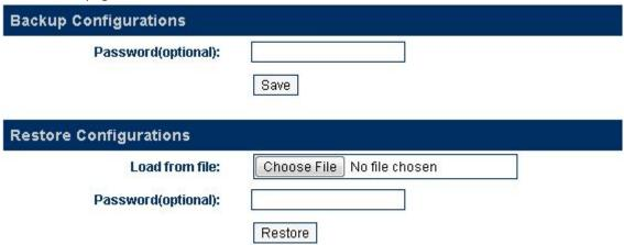
To backup the device configuration, just click [Save] in the Backup Configuration section. If a password is required when restoring a saved configuration, enter a password before the backup.
