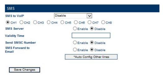
This page covers parameters that are related to SMS. The top parameter (SMS to VoIP) is a general setting for all channels. This defines how received SMS messages are used for Call Back or Forward functions which are described in details in the table below.
