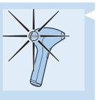
The 'ready to flash' light on the back of the appliance lights up green when all contact switches of the safety ring are in contact with the skin and the device is charged. This may take up to 3.5 seconds.
