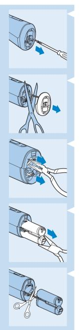
2 Undo the two screws in the bottom of the handle with a screwdriver.
