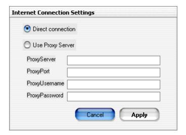
Direct connection - This is selected by default and is used when you have a direct internet connection. Use Proxy Server - Select this option if you are behind a Proxy Server. Enter the Proxy Server address and the Port. Also the Proxy Username and Password should be entered if it is applicable. Please consult your network administrator about information about your Proxy Server.
