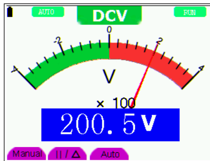
Figure 25: DC Voltage Measurement
