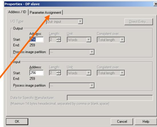
After choosing the „Device-specific parameters“ the different parameters (depend on the encoder version) can be set. If several possibilities are offered for one parameter the parameters list is opened by
