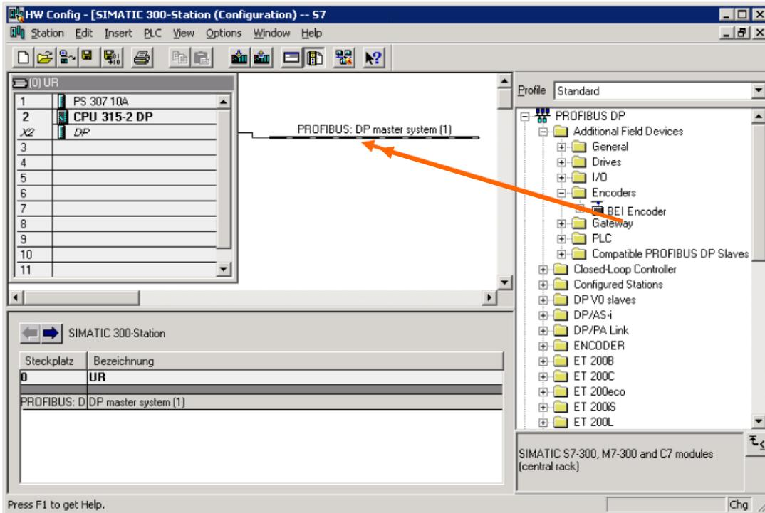
After inserting the Profibus master system in the hardware configuration ("Insert" – "Master System") the BEI IDEACOD encoder can be chosen from the hardware catalogue and added to the profibus network: Select the device "BEI IDEACOD Encoder" and drag it with the mouse to the network (or choose the network and double click the "BEI IDEACOD encoder").
