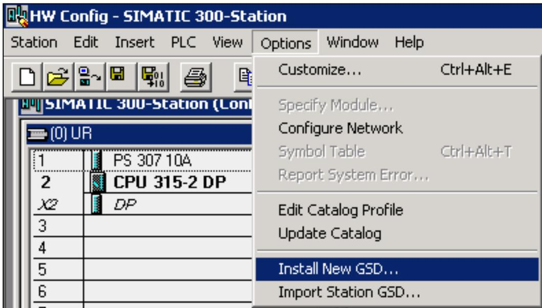
After the successful installation of the GSD file the BEI IDEACOD encoder can be found in the hardware catalogue under „PROFIBUS-DP“ – „Additional Field Devices“ – „Encoders“ – „BEI IDEACOD Encoder“.
