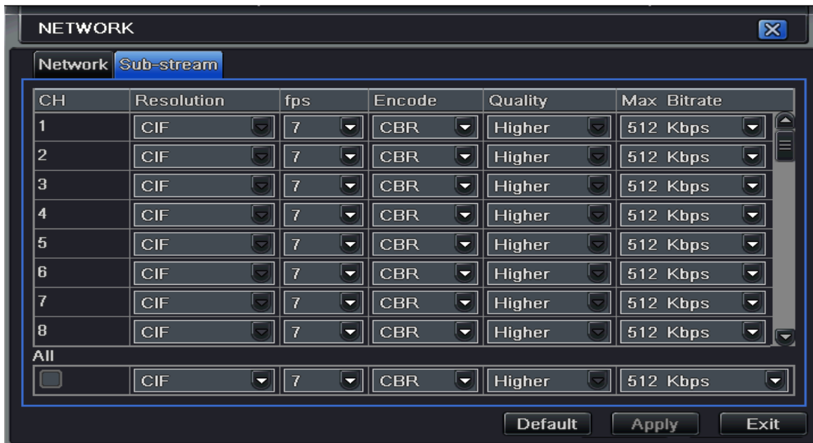
(10) Fig 4-33 network configuration-sub stream (11)
