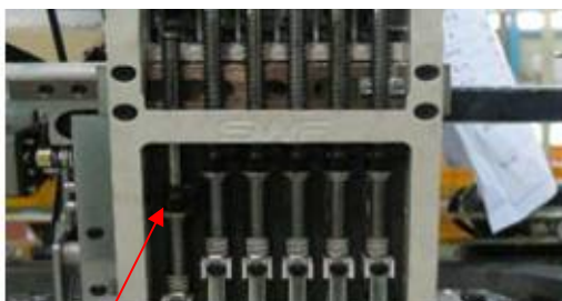
fix needlebar holder bolt after lifting up needlebar holder.
