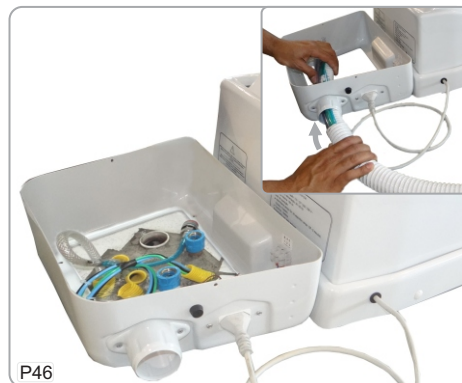
46-Place Junction Box over all connections and pass the hoses through the connector (detail).
