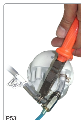
53-Connect the hose from Saliva Ejector drain.
