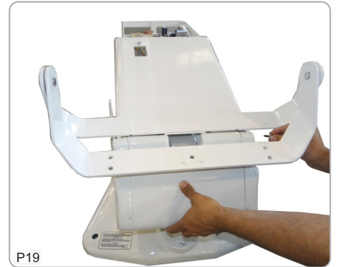
P19 19-Remove the rear pantograph cover and keep the four screws.
