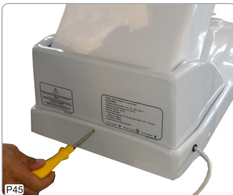
45-Remove the front plastic cover of the pantograph using a Philips screwdriver.
