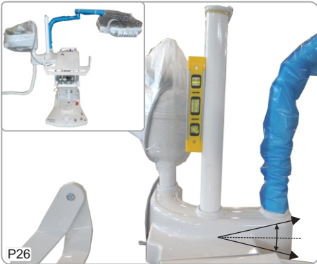
P26 26-Put the Working Table at working position and fix magnetic level on the post of Operating Light.
