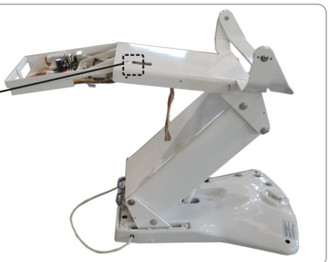
22-Release the counter nuts above indicated using two 13mm wrenches. Thread up the top nut (touching the metal plate). Remove the lower nut from the screw and keep it.
