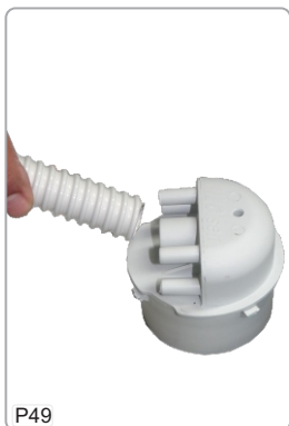
49-Connect the hose from cuspidor drain.
