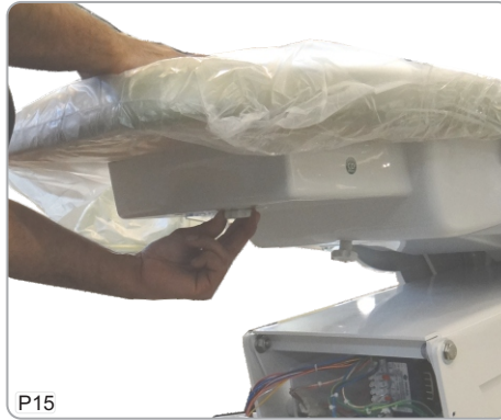
P15 15-Release the seat fixing handle screw.
