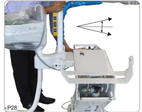
P28 28-Turn the magnetic level to adjust the delivery unit perpendicular level to the chair.
