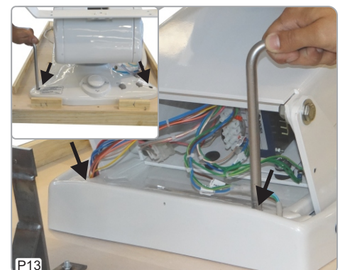
P13 13-Remove the chair fixing screws using L Wrench 11mm.
