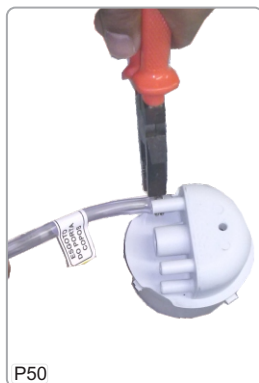
50-Connect the hose from cup-filler drain.
