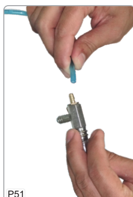
51-Connect the hose from air to the venturi saliva ejector.
