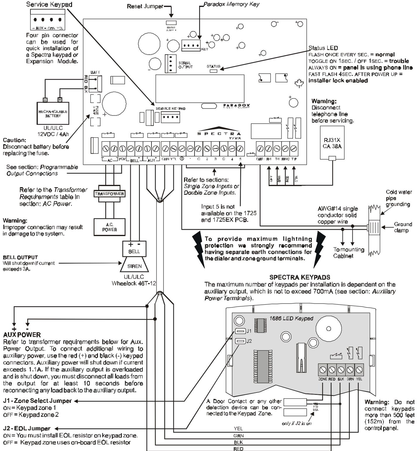
**Figure 2-1B: Spectra 1758 and 1758EX Control Panel Overview**
