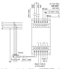
\* Dual voltage supply only available on 115/230 VAC model. For Us = 115VAC, connect the supply to terminals 6 and 7. For the other supply options, cable between 5 and 7.
