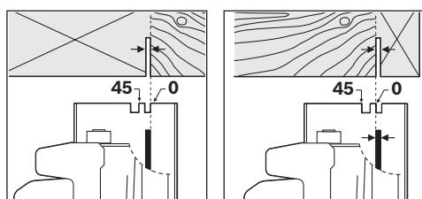
The 0° cutting mark (11) indicates the position of the saw blade for right-angled cuts. The 45° cutting mark (10) indicates the position of the saw blade for 45° cuts.
