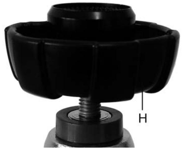
6. Place the handwheel **H** upside down on the double flats of the valve spindle.
