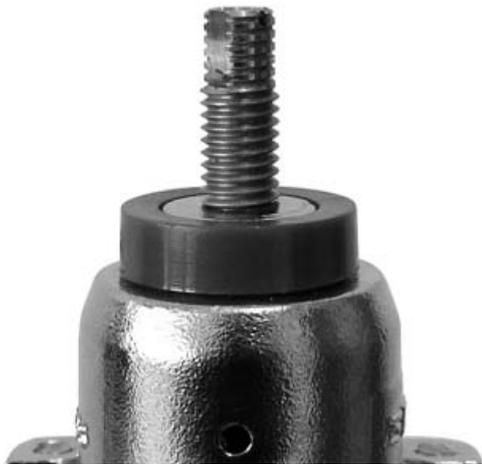
5. Dependent on the operating conditions, regrease the threaded spindle, especially a valve that is autoclaved.
