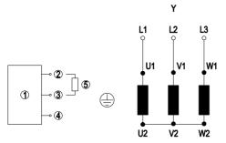
Changing the direction of rotation by reversing the two phases
