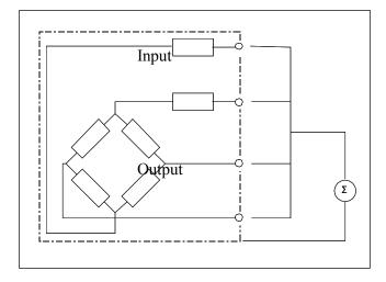
load cell or cable. Extremely low values ( $\leq 1k~\Omega$ ) indicate a short circuit rather than moisture ingress.
