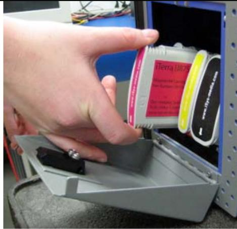
Match the color of the cartridge to the slot in the printer. Insert the cartridge until it clicks into place. As the ink cartridges are inserted, the front panel will display the ink levels.
