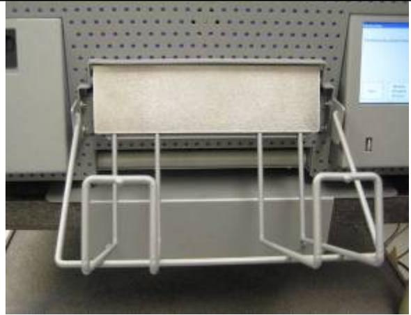
The output basket should be attached to the front of the printer as shown in the image above.
