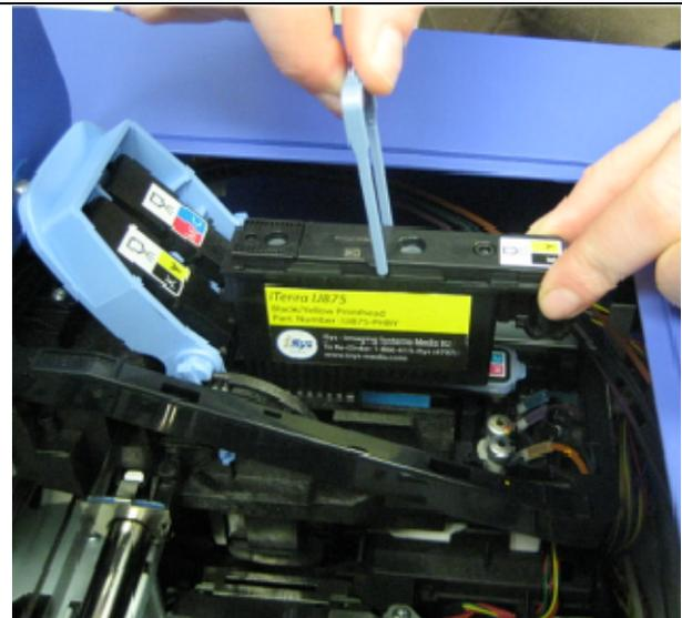
Lift the blue cover and press the printheads firmly into their appropriate slots so they click into place, returning the blue printhead handle to its lower position.
