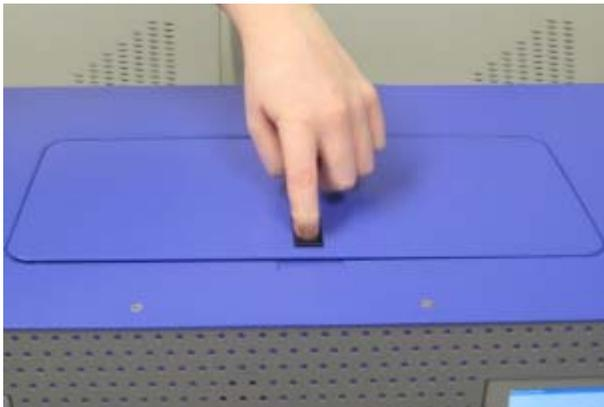
Push the black latch down to open the hinged printhead cover located at the top of the printer.
