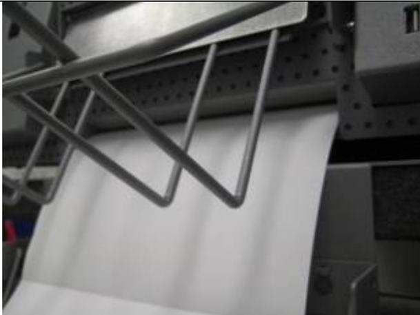
Start on a face up, non I-mark sheet of paper, press the form feed button and feed the end of the paper into the printer until the printer automatically takes the paper.
