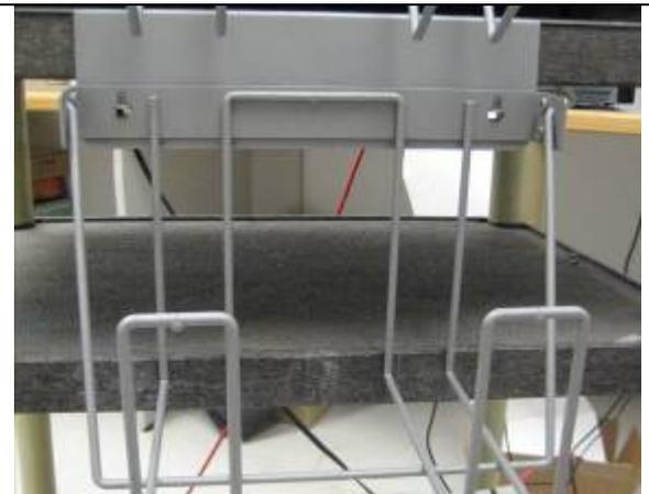
The input basket should be attached to the front of the plate as shown in the image above.
