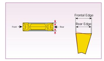
The HELIFACE twisted insert body shape makes it possible to machine deeper than insert length. The rear cutting edge slants in relation to the frontal cutting edge and does not make contact with the groove surface. The double prismatic clamping surfaces guarantee stability in seat and efficient side-turning options.
