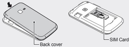
2. Insert the battery and replace the back cover.
