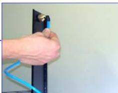
5) fix the flex tube LDA5 in the external side of the syringes holder tower.
