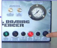
2) Unlock the pressure regulator (B) , now you can add or release pressure.
