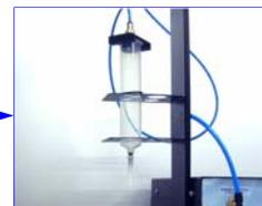
10) Connect air to the dispenser using the fast plug included.
