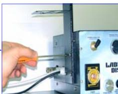
3) Put the blue tube blue ( biggest ) into the air tube socket (L) on the unit
