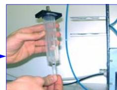
8) Fix the tube VMA5 in the aluminium syringes connector LDA3 .
