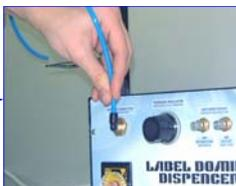
4) Put the blue tube blue ( biggest ) in the internal side of the syringes holder tower.
