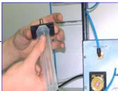
7) Fix the needle LDA1 with cap in the syringe LDA2 .
