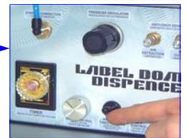
12) Regulate the pause time (F) and you'll only move between labels keeping pushed the foot-pedal.
