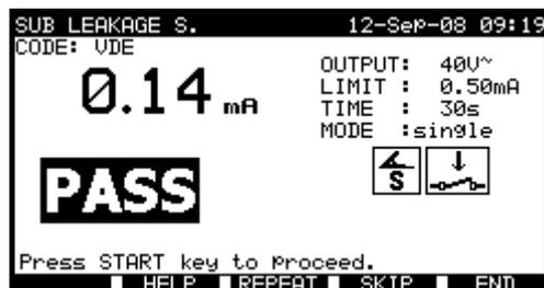
*Substitute leakage current measurement - Class II***Notes:**
