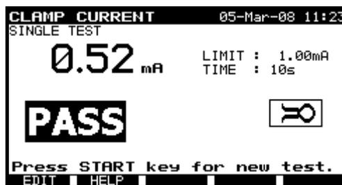
*Example of clamp current measurement result*
