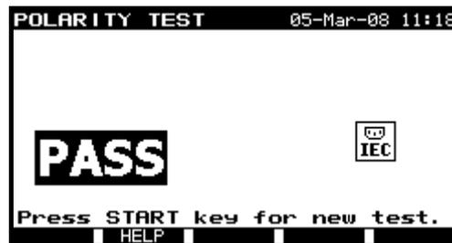
*Example of polarity test result*
