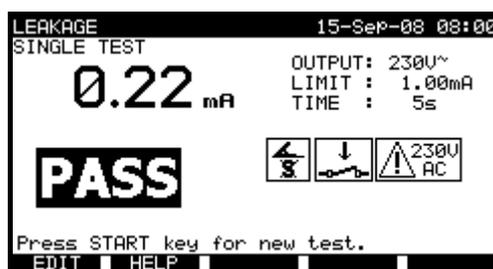
*Example of differential current measurement result*
