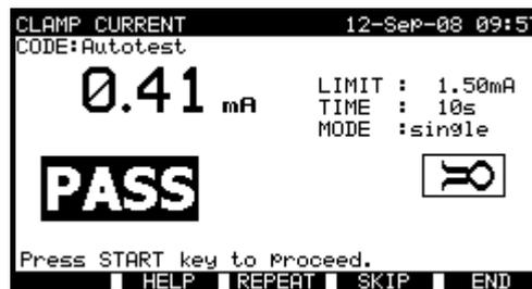
TRMS current measurement using current clamps
