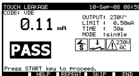
Touch leakage current measurement
