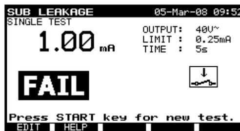
Examples of substitute leakage current measurement results
