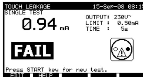
Examples of touch leakage current measurement results (slika)
