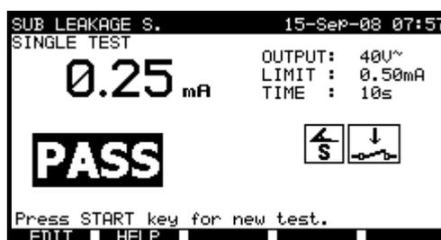
Example of substitute leakage current measurement results
