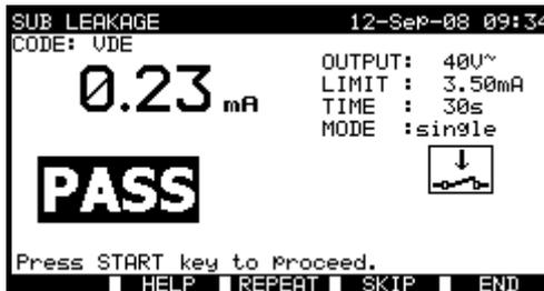
*Substitute leakage current measurement*
