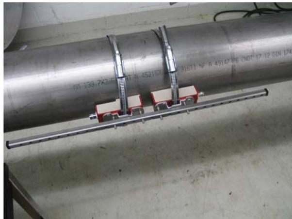
Illustration 4: Example of the V mode with mounting rail
