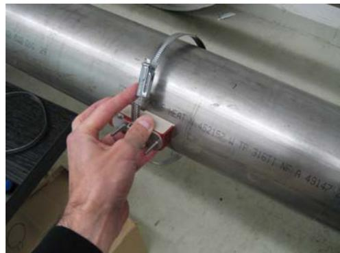
**Illustration 11:** Threading up the mounting belt
