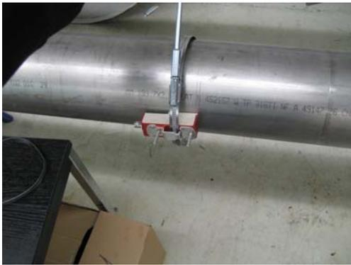
Illustration 12: Tightening of the mounting belt with the tightener
