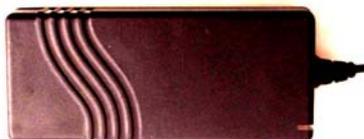
The power supply unit is usually used to load the rechargeable battery. It is of course also possible to use it for a continuous mains supply of your PortaSonic 9000.
