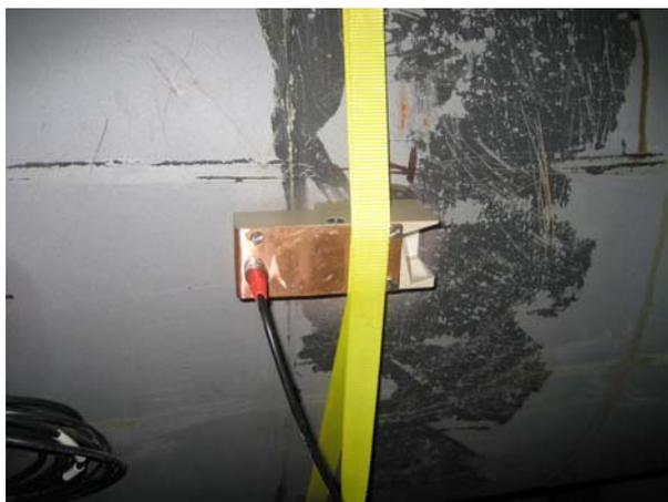
**Illustration 5** Ultrasonic sensor for large pipelines – textile mounting belt for the sensor mounting
