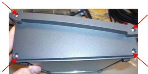
Remove the display and the keyboard from the lower part of the housing.
