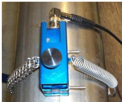
**Illustration 6:** Fixing the ultrasonic sensor (type F10, F20) by means of a stainless steel span chain
