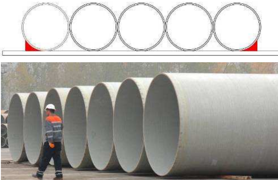
Figure 4: Storage of pipes as a single level
