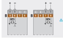
When terminals 5, 6 and 7, 8 are not configured as OP3 and OP4 outputs, they can be used as voltage or isolated contact inputs.
