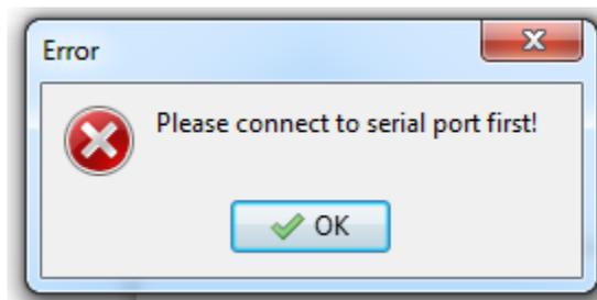
If the FMS interface does not answer to the commands, the following window will appear. Please reset the FMS interface, select another serial port or try the 'AUTO detect' button.
