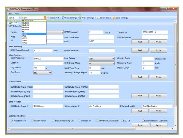
Select the correct Com number according to the Device Manager and select tracker's model. And then click the 'Open Port' button.
