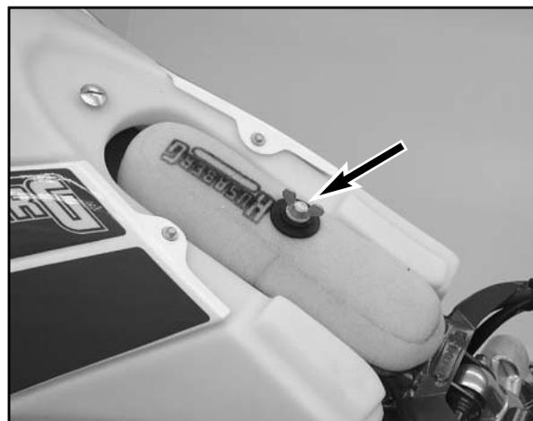
Thoroughly wash the air filter with special cleaning fluid and allow to dry. Press out the water from the air filter but do not wring. Lubricate the dry air filter with high-grade filter oil. Check the carburetor connection boot for damage and a good fit.
