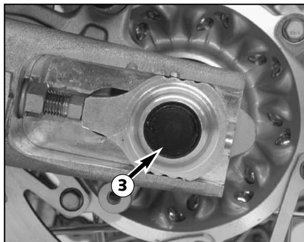
The rear wheel is remounted in the reverse order. Before tightening the collar nut to 80 Nm, push the rear wheel forwards so that the chain tensioners lie on the tension screws.
