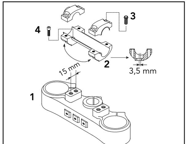
**WARNING:** The screws (4) must be secured with Loctite 243.
