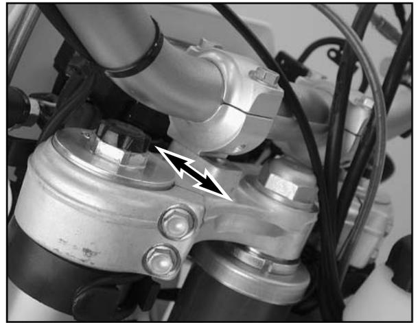
For this purpose, remove screws (3) of the handlebar clamps and screws (4) of the handlebar support. Position the handlebar support, and tighten screws (4) to 40 Nm. Mount handlebar and handlebar clamps, and tighten screws (3) to 20 Nm. The gap between the handlebar support and the handlebar clamps should be the same in the front and in the rear.
