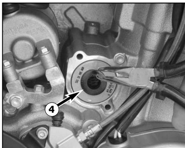
Lay the motorcycle down and fill the oil filter housing approx. half-full with engine oil. Insert the oil filter in the housing. Grease the O-rings in the oil filter cover and mount the cover. Mount the screws and tighten to 6 Nm.
