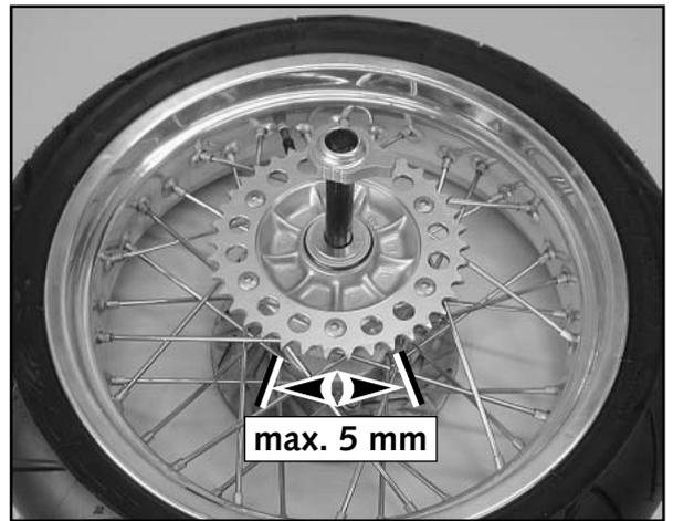
For this purpose, lie the rear wheel on a work bench with the rear sprocket upwards, and put the wheel spindle in the hub. Now hold the rear wheel firmly and try to turn the rear sprocket. The rear sprocket may not turn more than maximum 5 mm (0,2 in) measured on the outside. If the play in the chain wheel is larger, all 6 shock absorption rubbers are to be replaced.
