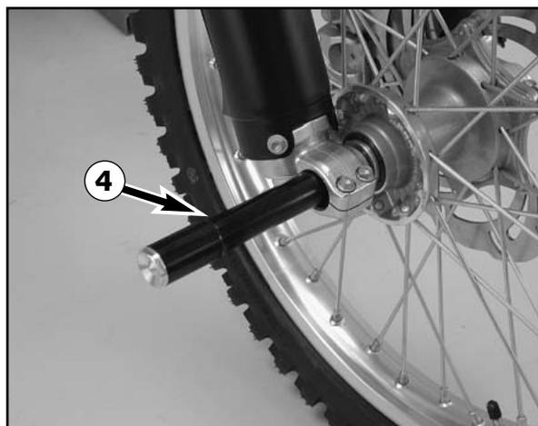
Before remounting the front wheel, clean and grease the shaft seal rings (A) and the bearing surface (B) of the distance bushings and mount the distance bushings
