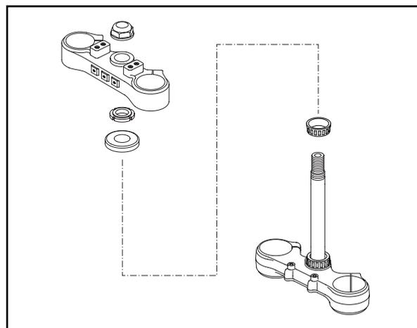
The steering head bearings should be regreased at least once a year (e.g. Motorex Long Therm 2000).
