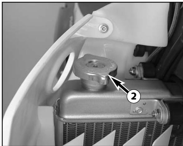
A mixture of 40% antifreeze liquid and 60% water is used as coolant. However, the antifreeze protection must be at least -25° C (-13° F). This mixture offers antifreeze protection but also good corrosion protection and should therefore not be replaced by pure water.
