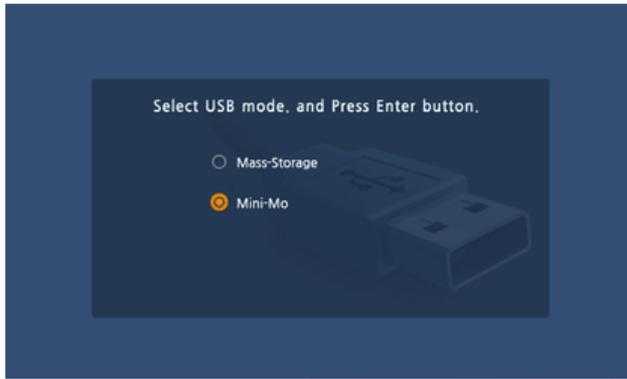
**MINI-MO is a function that enables the Digital Photo Frame to be operated as the Secondary Monitor.**
