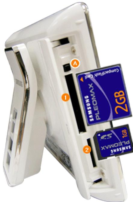
**1 CF CARD** Slide the card into in the direction marked on the top of the card. To remove a memory card, press **A** the button at the top of the card slot.
