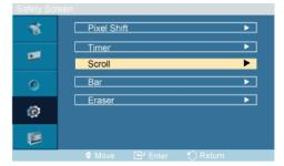
This function helps to remove after-images on the screen by moving all the pixels on the LCD according to a pattern.
