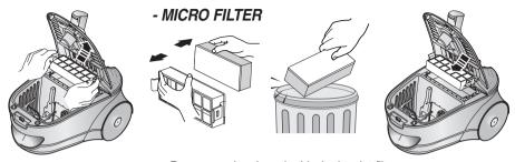
Remove and replace the blocked outlet-filter.
