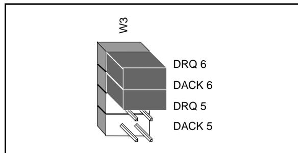
Figure 2-8. DMA Channel Jumper Setting for DMA Channel 6
