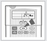
2 To select the HEAT mode, press the button until is displayed at the top of the wired remote controller.
