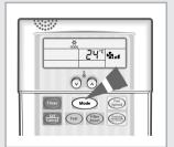
2 To select the COOL mode, press the button until is displayed at the top of the wired remote controller.
