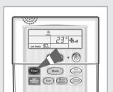
The Off Timer enables you to switch off the air conditioner automatically after a given period of time. You can set the period of time from 30 minutes to 24 hours. You can select the Off Timer only when the air conditioner is on.
