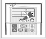
4 Select the fan speed by pressing the button one or more times until the intended value is displayed:
