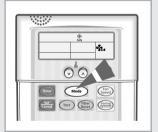
2 To select the FAN mode, press the button until is is displayed at the top of the wired remote controller.
