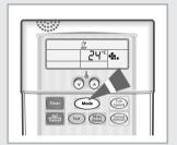
2 To select the DRY mode, press the Mode button until is displayed at the top of the wired remote controller.
