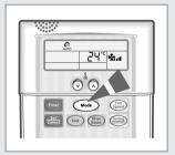
2 To select the AUTO mode, press the button until surply is displayed at the top of the wired remote controller.
