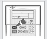
The On Timer enables you to switch on the air conditioner automatically after a given period of time. You can set the period of time from 30 minutes to 24 hours. You can select the On Timer only when the air conditioner is off.
