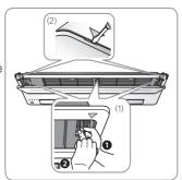
Pull out the Air filter. Grab the Air filter and lift it upwards while pushing slightly, and then pull the Air filter forward.
