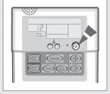
To select the AUTO mode, press the Mode button until is displayed at the top of the function controller.
