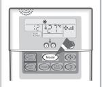
2 To select the COOL mode, press the Mode button until is displayed at the top of the function controller.
