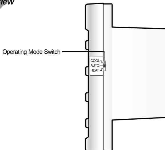
**Note** ♦ Choose the appropriate operating mode with the Operating Mode Switch that enables the user to choose between the Cool/Auto/Heat mode.
