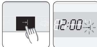
2. Turn the **Time / Temp Control Dial** to set the desired end time.
