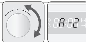
4. Select the desired weight by turning the **Time/Temp control dial** to the right and left. Preheating time(min:sec) is displayed, and countdown starts 5 seconds after the weight is selected. For a recipe without preheating, remaining cooking time(hr:min) is displayed.
