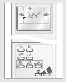
The air conditioner can generate anions with an ionizer in the indoor unit. Since it is an additional function, you can select it any mode, even when the air conditioner is turned off.
