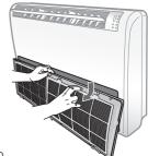
**4.** Clean the Air filter with a vacuum cleaner or soft brush. If dust is too heavy, then rinse it with running water and dry it in a ventilated area.
