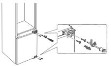
4. Remove the screws from the refrigerator. Disassemble the freezer door and hinges.
