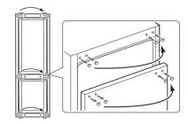
**EXAMPLE** Be careful not to get injured while removing the Screw cap.
