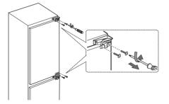
2. Remove the screws from the refrigerator. Disassemble the fridge door and hinges.
