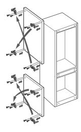
7. Tighten the screws on the refrigerator.
